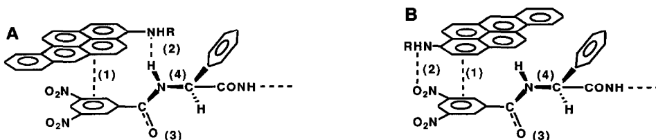
Fig. 3. Proposed three-point interaction model between Pirkle-type chiral stationary phase and the best orientations of 3-aminobenzo[a]pyrene (panel A and panel B) for maximum interaction. The number in parenthesis represents the type of interaction, as described in the text.
